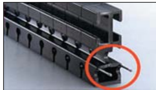
Steel cables extruded directly into the carrier sidebands significantly increase carrier system tensile strength and can be used to monitor carrier wear
